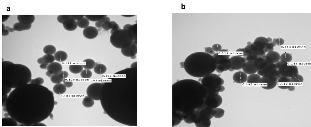
**Figure 3:** TEM photographs of (a) SF@NPs and (b) SF-3AQ@NPs.
