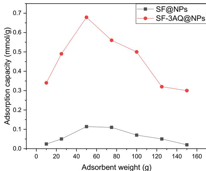
**Figure 8:** Effect of adsorbent weight on Pb(II) adsorption capacity using SF@NPs and SF-3AQ@NPs adsorbents.
