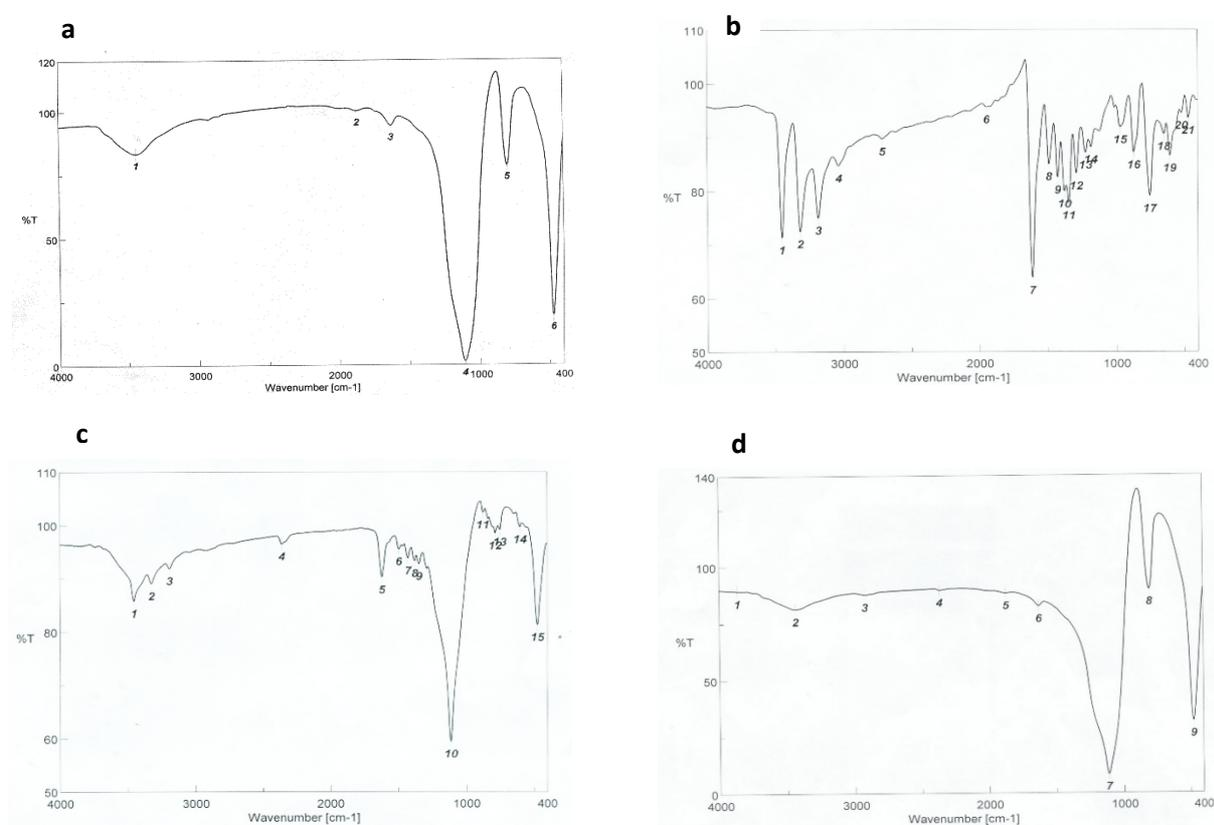
**Figure 1:** FT-IR spectra of Nano adsorbents: (a) SF@NPs (b) 3AQ, (c) SF-3AQ@NPs, and (d) SF-3AQ@NPs after adsorption of  $\text{Pb(II)}$ .
