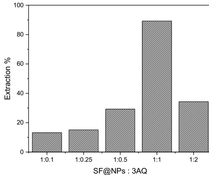
**Figure 5:** The extraction percent of the new modified SF@NPs composites for Pb(II) adsorption with different SF@NPs: 3AQ mass ratios
