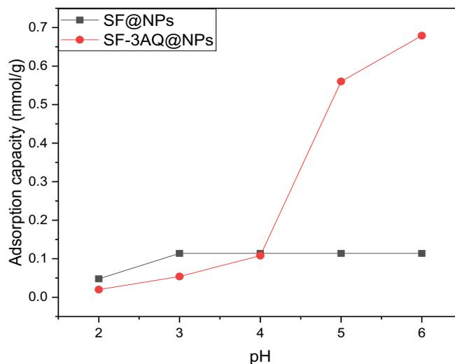
**Figure 6:** Effect of pH on Pb(II) adsorption capacity using SF@NPs and SF-3AQ@NPs adsorbents.
