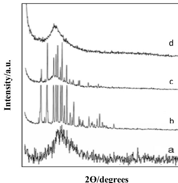
**Figure 2:** X-ray diffraction spectra of (a) SF@NPs, (b) 3AQ, (c) SF-3AQ@NPs, and (d) SF-3AQ@NPs after adsorption of Pb(II).
