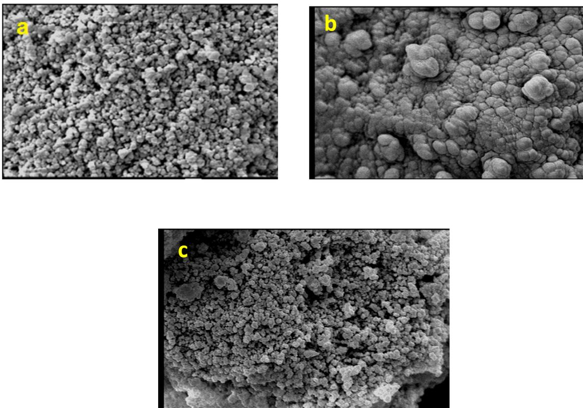
**Figure 4:** SEM photographs of (a) SF@NPs, (b) SF-3AQ@NPs, and (c) SF-3AQ@NPs after adsorption of Pb(II).
