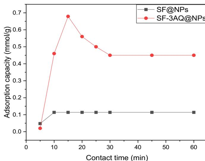
**Figure 7:** Effect of contact time on Pb(II) adsorption capacity using SF@NPs and SF-3AQ@NPs adsorbents.
